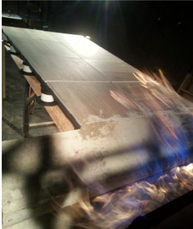
Photograph 3: Tile Tech Porcelain Paver Deck at Maximum Flame Spread (0 Feet)
