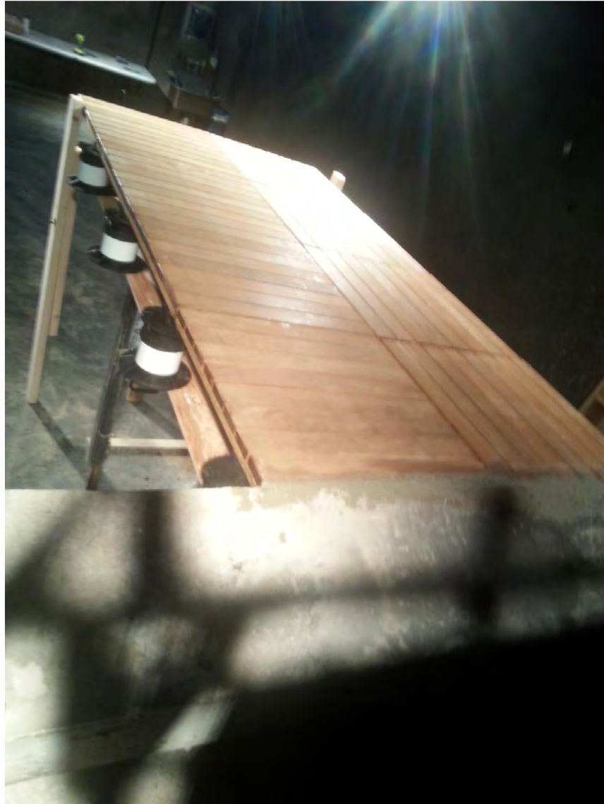
Photograph 1: Ipe Wood Tile Deck Prior to Testing
