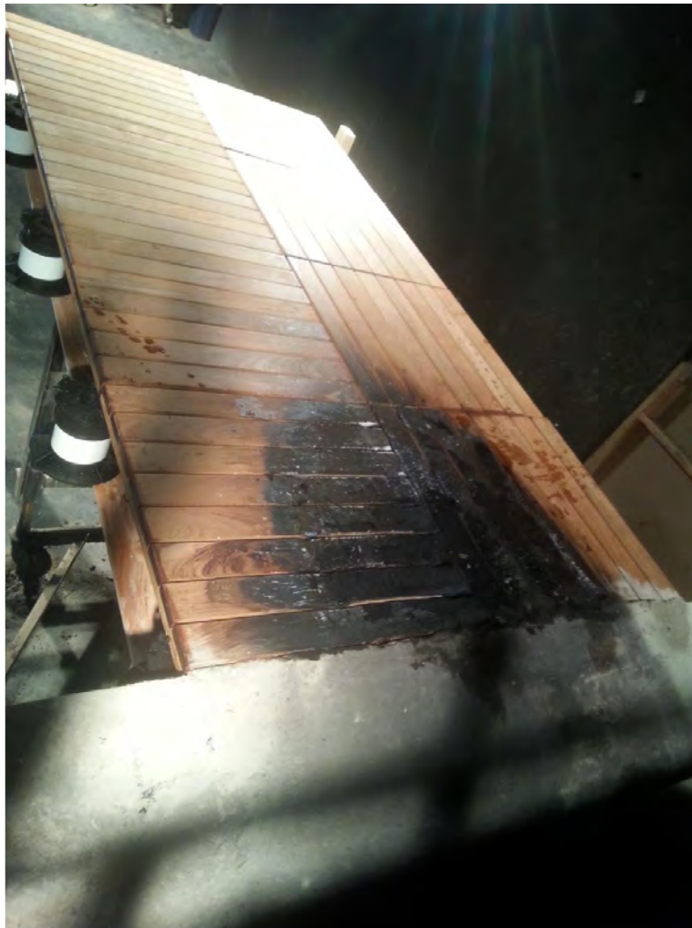
Photograph 3: Ipe Wood Tile Deck After Test Completion
